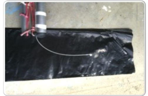
Tape nylon zip tie to end of upper spar for downwind tell.
