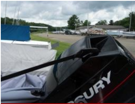
Above: Hook strap that goes through marks (barrels) on motor not on boat stern eyes like below
