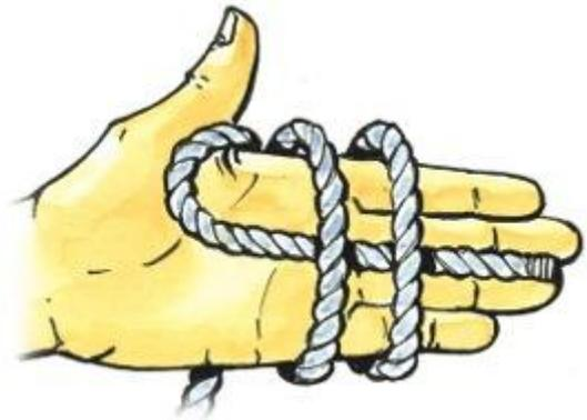
**Stopper Knot** - To keep a line from pulling through a block or rope clutch, a knot should be tied in the end of it. The most secure knot for doing this is the double overhand stopper knot, known as the stopper knot for short. Unlike a simple overhand knot or a figure eight knot, this knot does not come loose easily.
