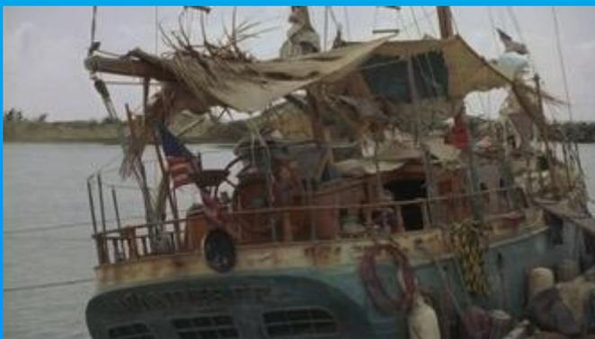
The *Wanderer* (the boat's real name) is an actual sailboat – a Formosan 51 ketch that is a sailing beauty. Teak everywhere and a sight to behold above and below deck. (A ketch is a two masted boat with the after or mizzenmast in front of the rudder post as opposed to a yawl which is the same thing but with the mizzenmast behind the rudder post. I had to look it up. Again.)
